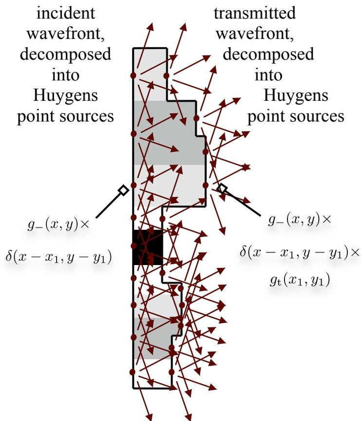
Using the sifting property of delta functions we can express the incident and transmitted wavefronts as
