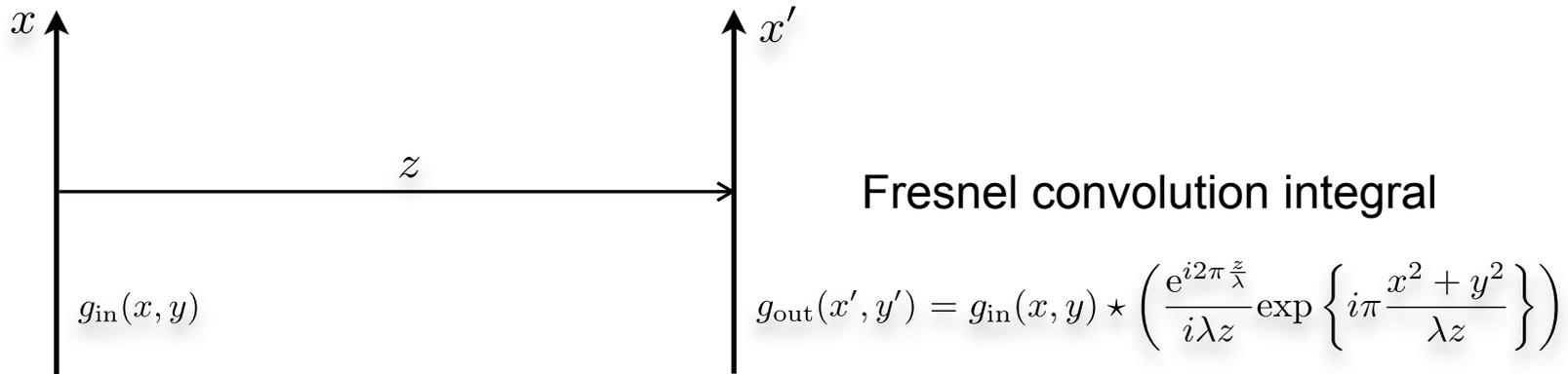
$$g_{\text{out}}(x', y'; z) = \frac{1}{i\lambda z} \exp \left\{ i2\pi \frac{z}{\lambda} \right\} \iint g_{\text{in}}(x, y) \exp \left\{ i\pi \frac{(x' - x)^2 + (y' - y)^2}{\lambda z} \right\} dx dy$$
