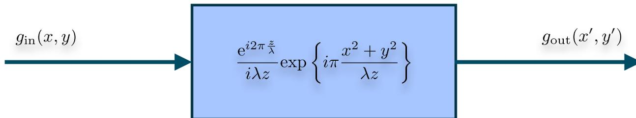
The spherical wave is the system's impulse response; in Optics, we refer to it as the **Point Spread Function (PSF)**.
