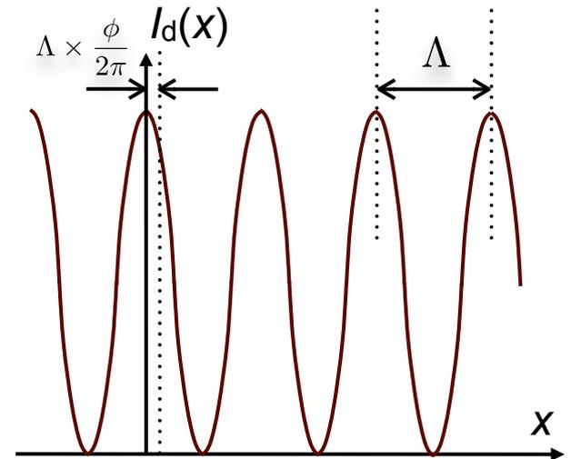
For example, consider a plane wave incident on the interferometer, with no unknown object (*i.e.* *clear object path*) and the signal mirror tilted by  $\theta$ .
