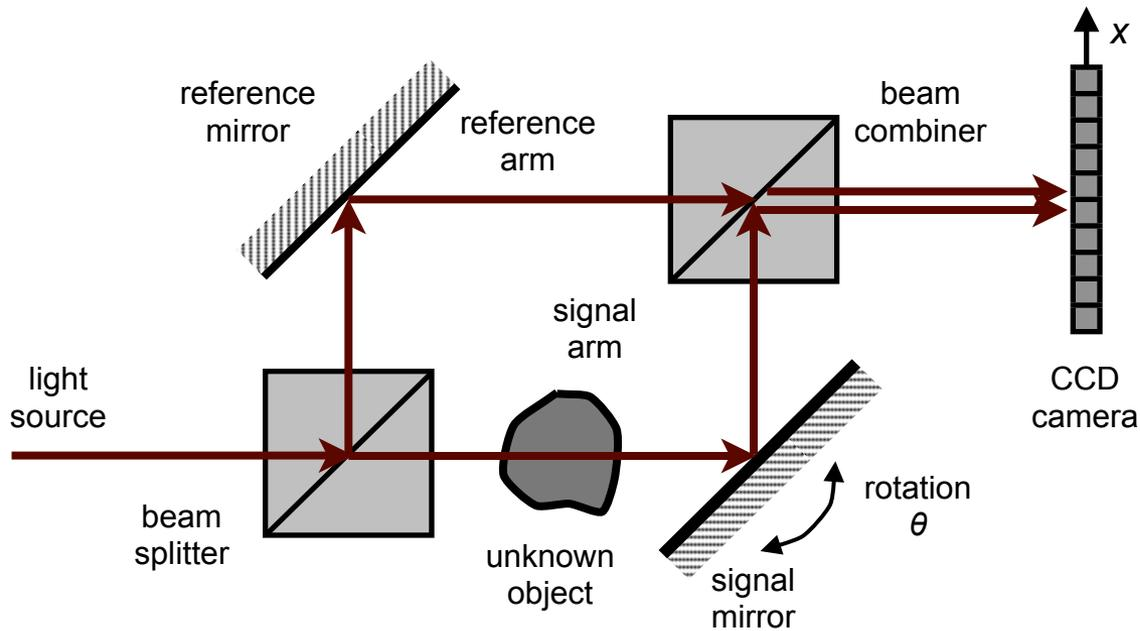
in this case the “interference pattern”  $I_d$  is function of position  $x$  so it is digitized by a pixelated sensor array (digital camera)
