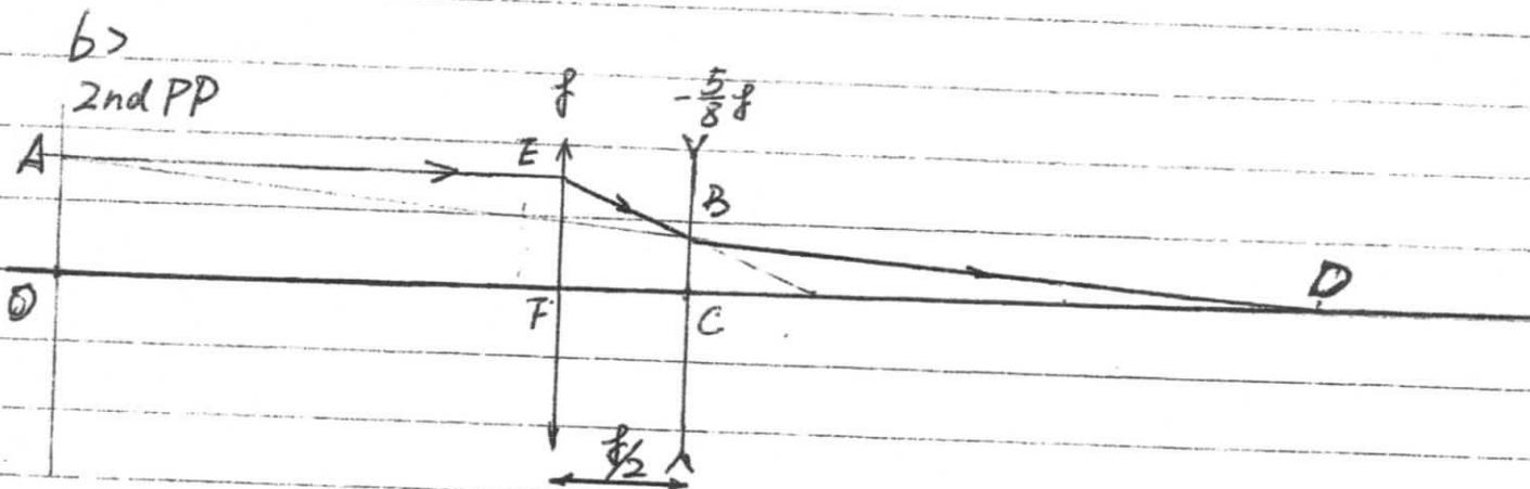
$$\overline{BC} = \frac{1}{2} \overline{EF} = \frac{1}{2} \overline{AO}$$
