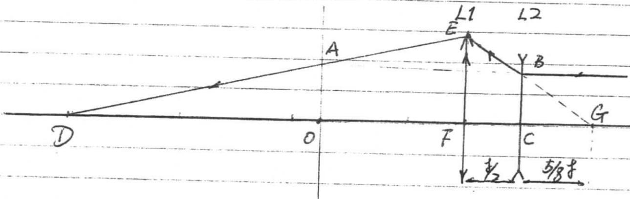
The parallel rays from left will have a virtual focal point at G after passing through Lens L2.
