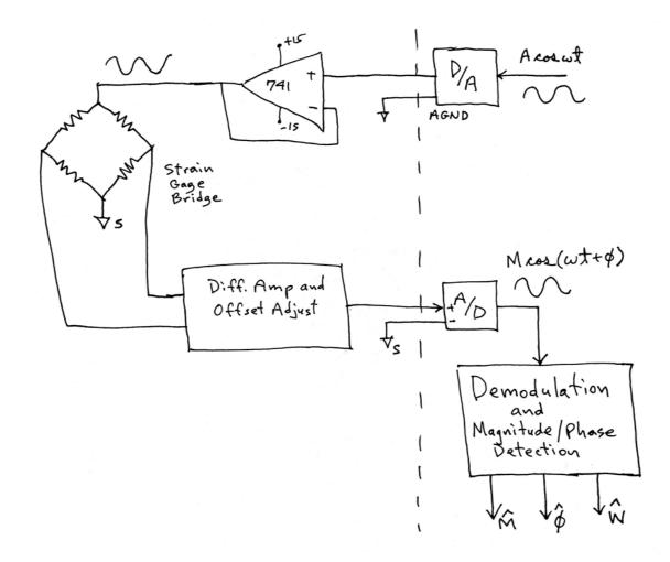
Figure 1: AC-driven and demodulated electronic scale circuit configuration.
