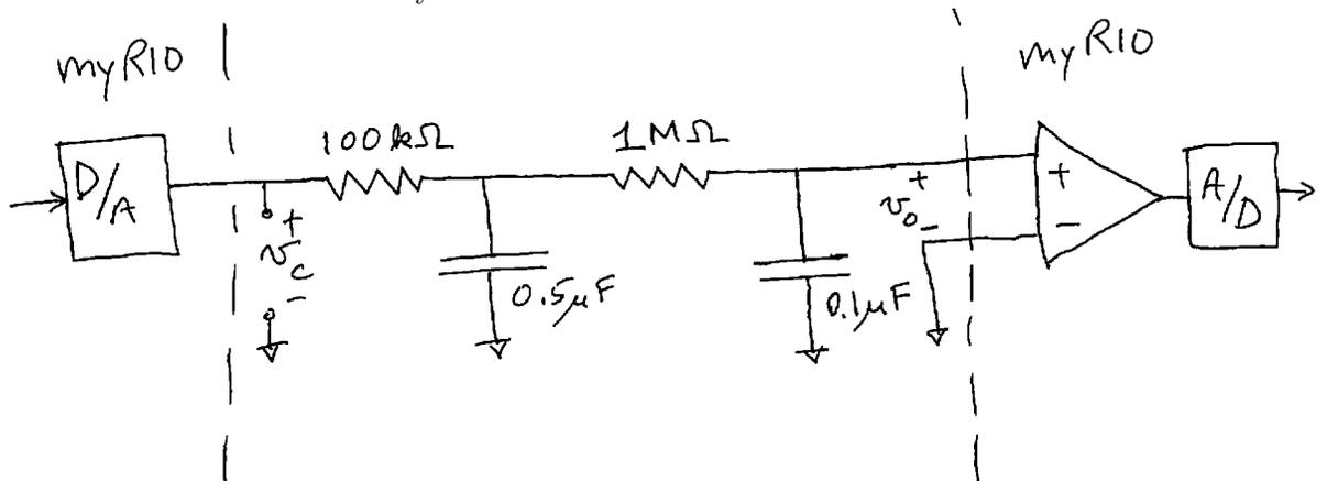
The second-order circuit shown is to be considered as the *plant* to be controlled by the myRIO. Specifically, the input to the plant is the D/A output voltage  $v_c$ , and the output of the plant is the voltage  $v_o$ . That is, the control loop configuration is:
