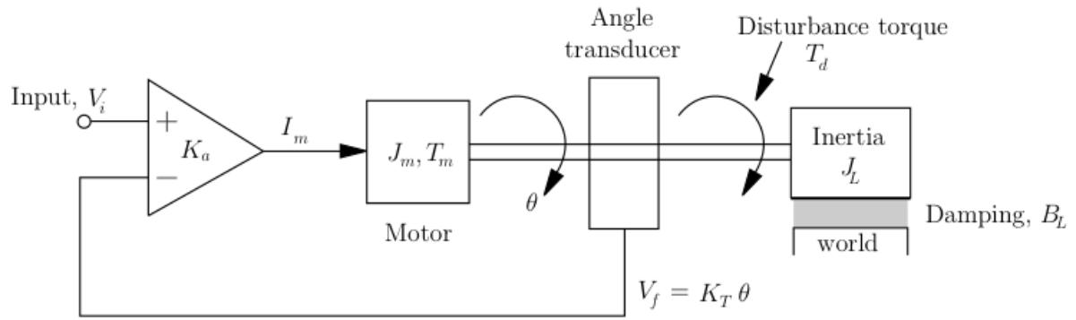
Figure 1.18: Servomechanism with an added disturbance torque.
