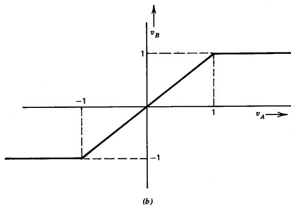
**Figure 2.22** Nonlinear feedback system. (a) System. (b) Transfer characteristics for nonlinear element.
