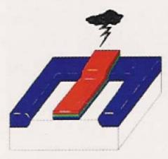
11. Polysilicon and a thin layer of silicon dioxide are removed by etching, exposing the underlying silicon substrate (white).
