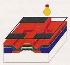
22. Light shining through the fourth patterned mask chemically changes the exposed photoresist.
