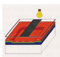
9. Light shining through a new patterned mask chemically changes the photoresist that is exposed to the light.
