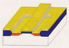
14. A new layer of silicon dioxide is deposited. It will insulate the transistor structure, except for metal contacts that will be added.
