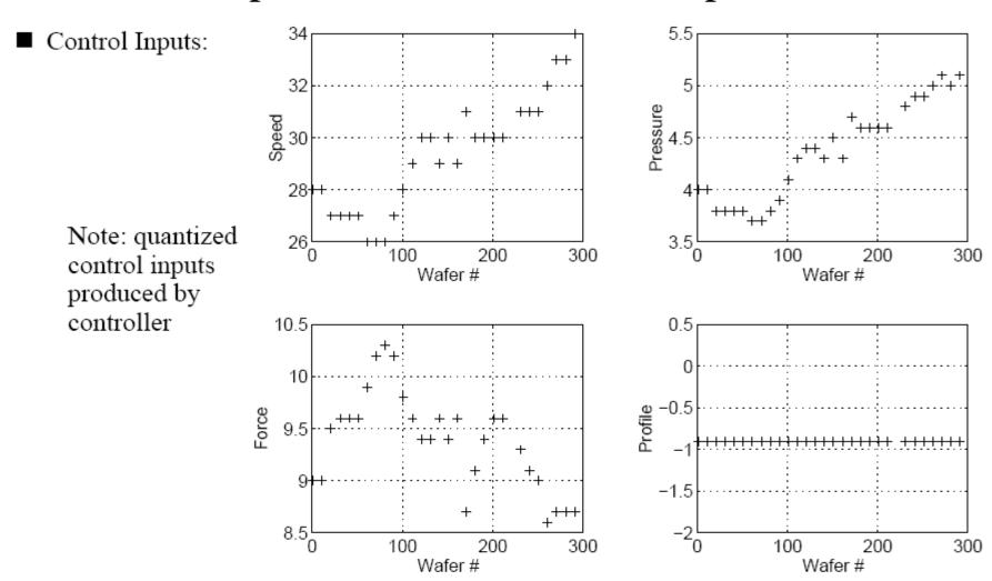
■ Controller produces increasingly aggressive control to compensate for drift
