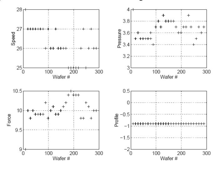
■ Control inputs have not hit any limitations: failure is in model update
