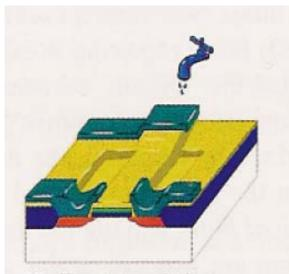
25. The photoresist is removed with a chemical solvent, completing the transistor. Many transistors are created simultaneously.
