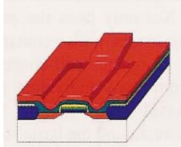
21. A fourth layer of photoresist is deposited on the wafer.
