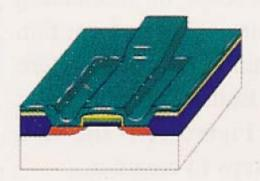
20. Aluminum (blue-green) is deposited over the surface and inside the three shafts. It will provide electrical connections.
