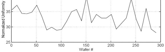
■ Controller successfully compensates for drift in the process
