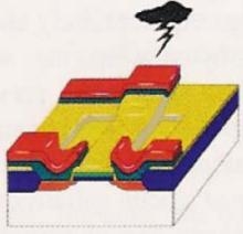
24. The exposed aluminum is etched away, leaving aluminum "wires" that will carry current to and from the transistor.
