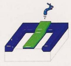
12. A chemical solvent washes away the remaining photoresist, leaving the polysilicon transistor gate structure (green).
