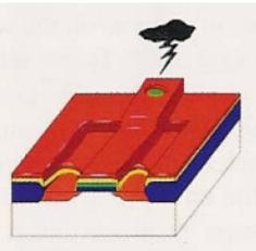
18. Dry etch removes the exposed silicon dioxide, opening shafts to the negatively doped substrate and the polysilicon.
