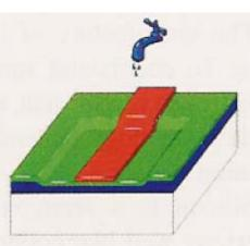
10. A chemical solvent removes the exposed photoresist, leaving a patterned layer of photoresist above the polysilicon.
