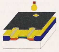
16. Light shining through a patterned mask chemically alters most of the photoresist, except three small areas for metal contacts.
