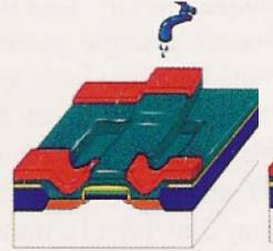
23. A chemical solvent removes the exposed photoresist, creating a photoresist pattern above the aluminum.
