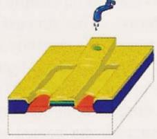
19. A chemical solvent removes the photoresist. The negatively doped source and drain (orange) and the polysilicon gate (green) are opened to metal contacts.
