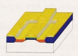
A layer of photoresist is deposited on the wafer, in preparation for metal contacts to the source, drain, and gate of the transistor.
