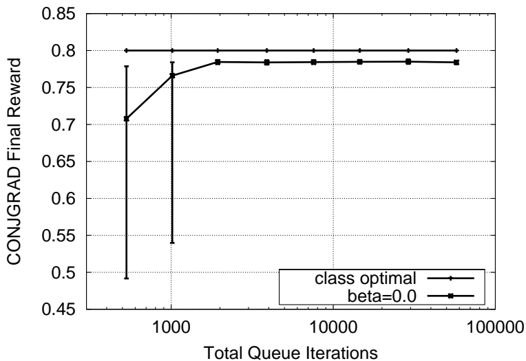
Figure 12: Performance of the call admission controller trained by CONJPOMDP as a function of the total number of iterations of the queue. The performance was computed by simulating the controller for 100,000 iterations. The average reward of the globally optimal policy is 0.804, the average reward of the optimal policy within the class is 0.8, and the plateau performance of CONJPOMDP is 0.784. The graphs are averages from 100 independent runs.
