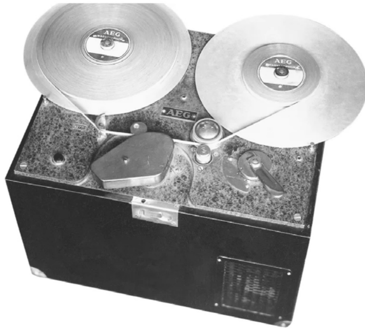
BASF's magnetic tape and AEG's magnetophone – the sensation at the Berlin Radio Fair in 1935
