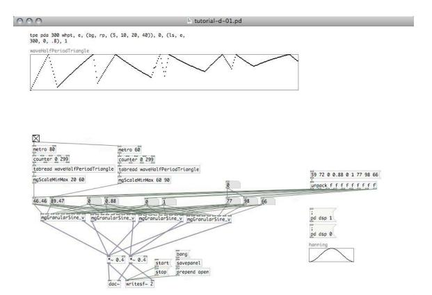
• Reading parameter values from multiple [tabread] and multiple tables at different rates
