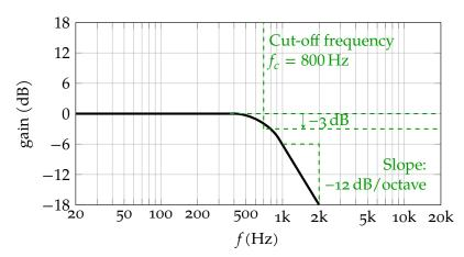
1. Which type of filter does the frequency response diagram above show?
