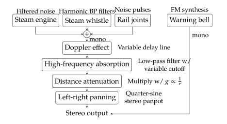
FIGURE 3. Block diagram of steam train drive-by model
