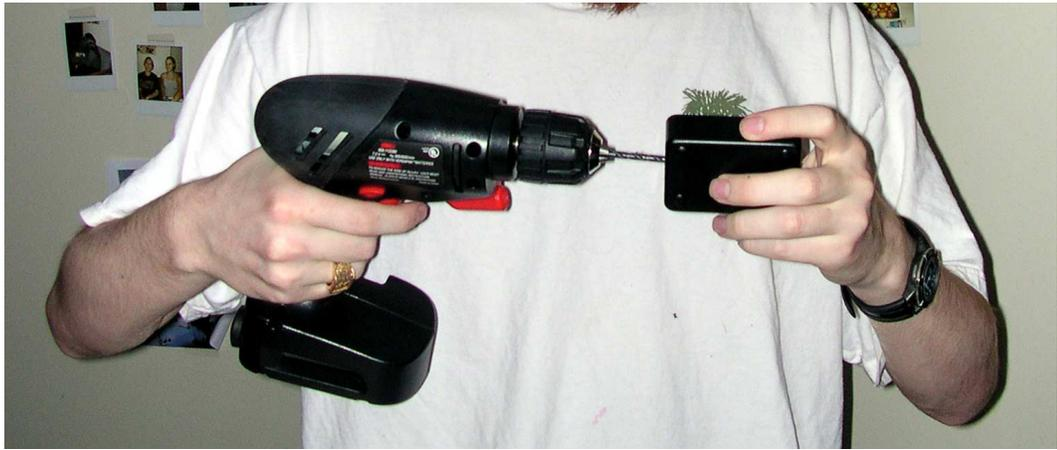
Figure 6: Drilling a hole in the enclosure
