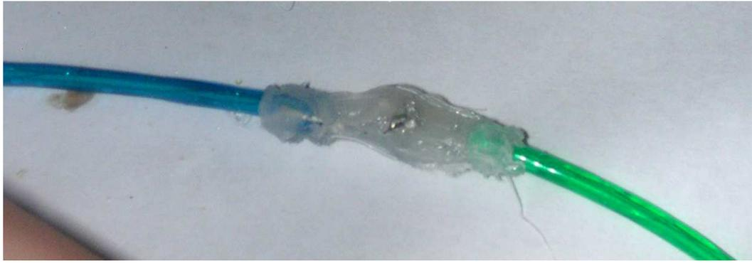
Figure 8: EL wire connection — glued
