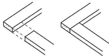
This must be attached with some other method of fastening, like glue or reinforcing sheets, as is common on flats. Though not inherently very strong, it is unbeatable for simplicity.
