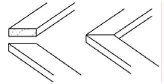
A miter joint is created by cutting the two pieces at supplementary angles, so the combined joint totals to 90 degrees. It has a better appearance than butt joint, as it doesn't expose the interior grain. This is slightly sounder than a butt joint, and it can be reinforced further by adding a lap (covered below) to form a half miter, or dowel pins or a tongue:
