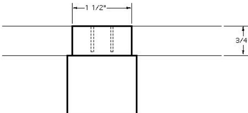
Our design involved quick modification of standard decorative candles so that the male plug extended immediately out of the base. These were mated with Edison female connectors mounted flush inside the lids of platforms in each location a candle was to be placed.
