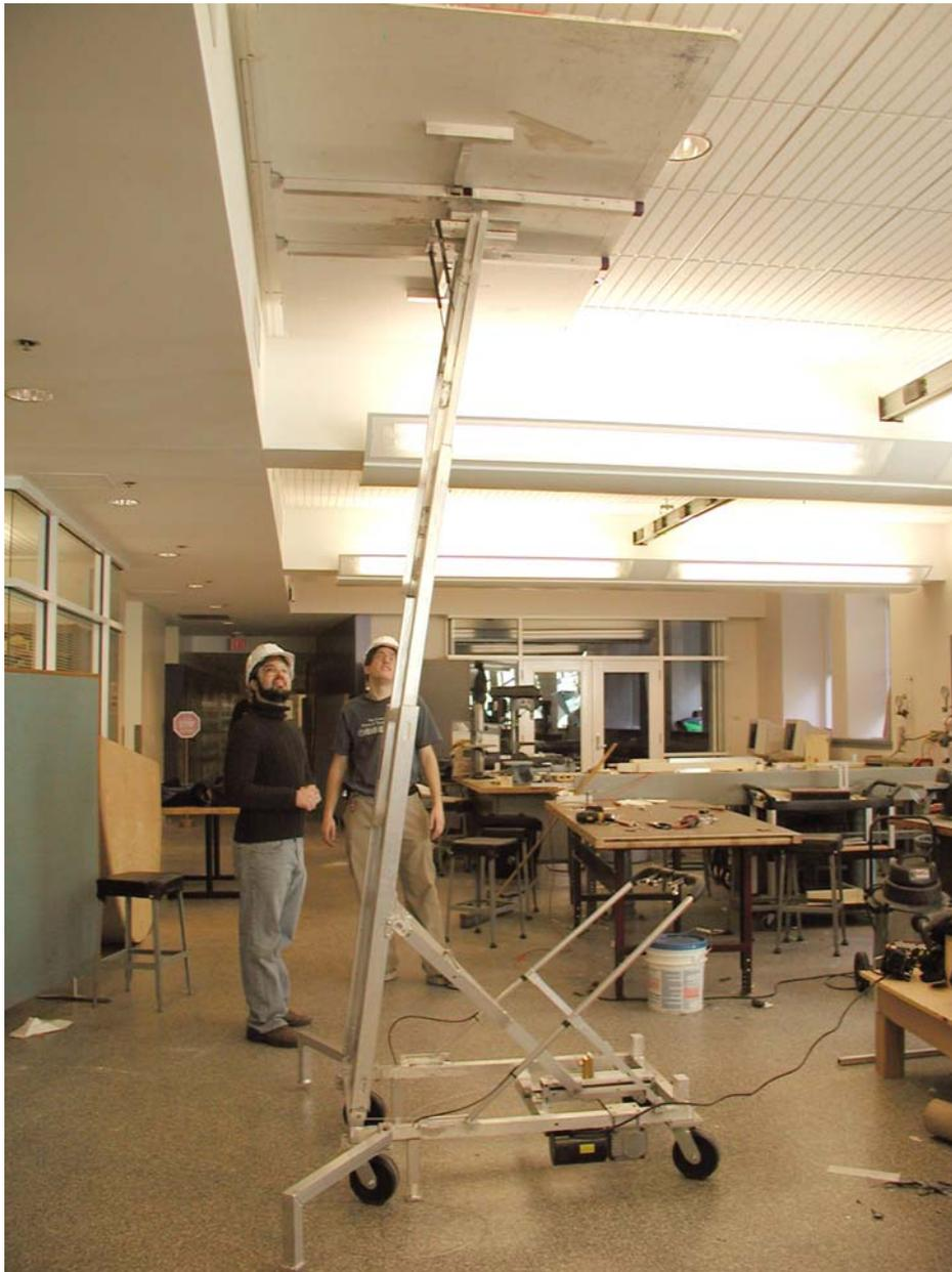
The drive mechanism is the small black motor seen attached to the base. The extensible lift was tilted slightly backward, so that as the drywall was lifted, it brought
