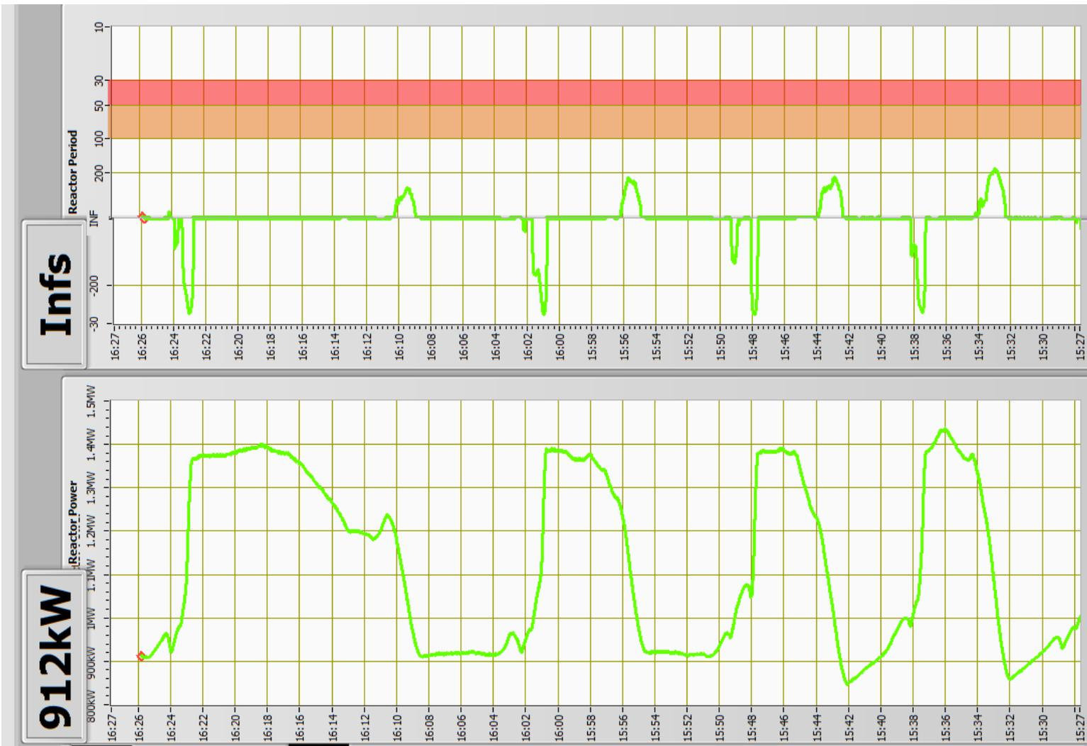
The graph on the bottom is the reactor power, while the graph on top is the “reactor period,” which is the mean time that it would take for the reactor to increase in power by a factor of  $e$ . There are a few features to notice here:
