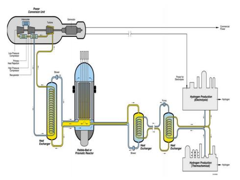
Figure 1. VHTR with electricity and hydrogen production alternatives.
