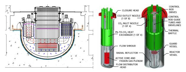
Figure 5. LFR options: ELSY (600 MWe) left, and SSTAR (20 MWe) right.
