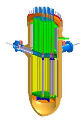
Figure 3. SCWR pressure vessel baseline alternative.<sup>3</sup>
