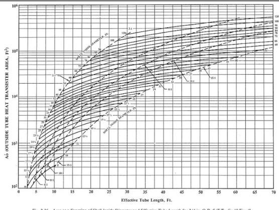
Fig. 2.26 Area as a Function of Shell Inside Diameter and Effective Tube Length for 3/4 in. O.D. S/T Trufin 19 Fins/In. on 15/16 in. Equilateral Triangular Tube Layout Fixed Tube Sheet, One Tubeside Pass, Fully Tubed Shell.
