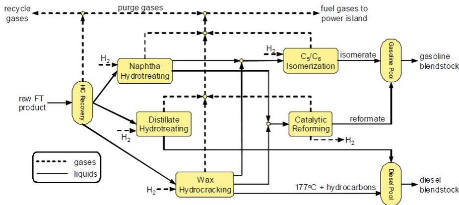
Figure 10: Schematic of FTL refining process
