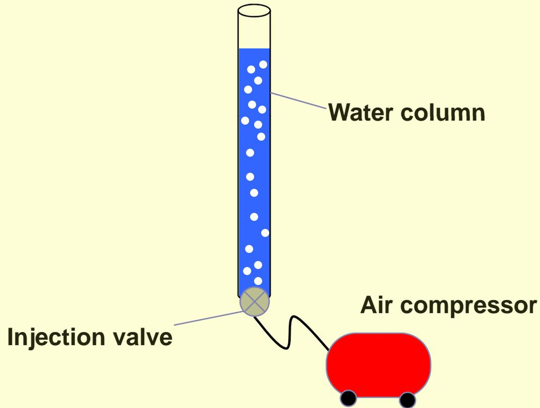
Watch how the flow pattern changes as air flow is increased
