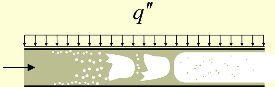
Saturated boiling in most of the channel
