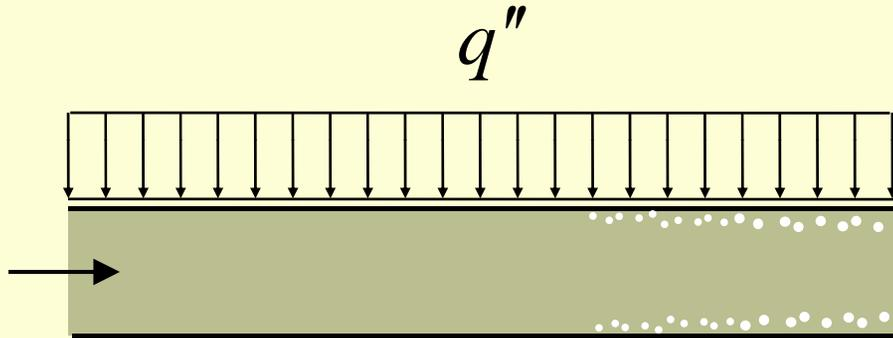
Subcooled boiling in the hot channel
