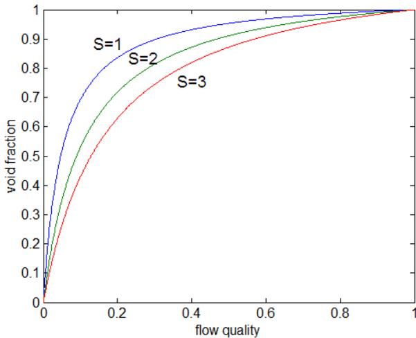
Figure 1. Effect of S on  $\alpha$  vs x for water at 7 MPa.
