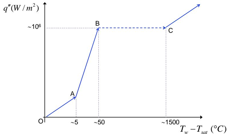
Figure 5. Qualitative boiling curve for water at atmospheric pressure ( $T_{sat}=100^\circ C$ ) on a flat plate.
