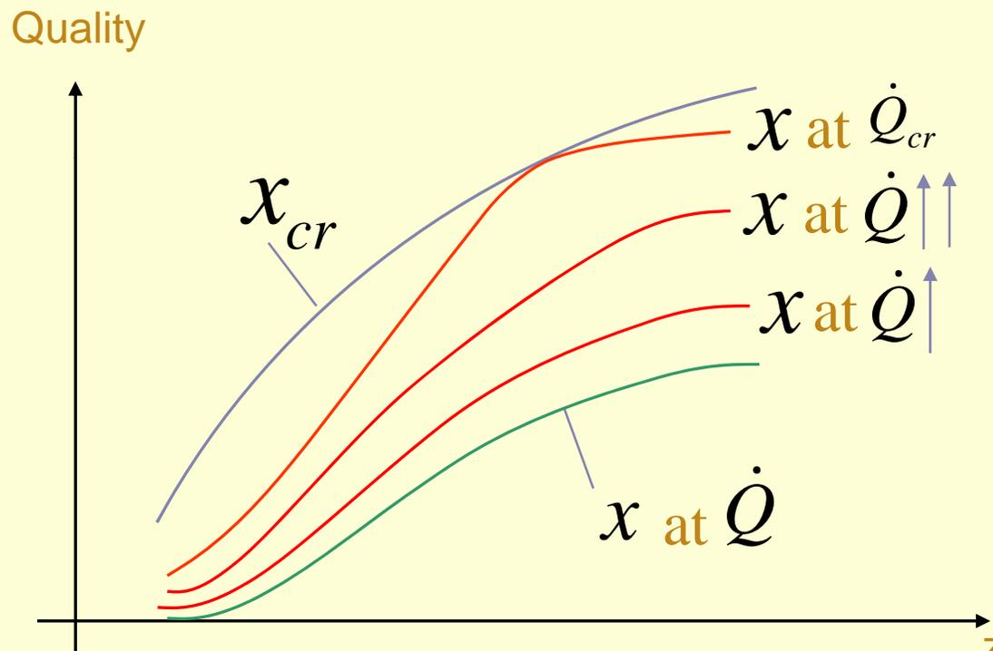
$$\text{Critical Power Ratio (CPR)} \equiv \frac{\dot{Q}_{cr}}{\dot{Q}} \quad \text{CPR} > 1.2 \text{ in the US}$$
