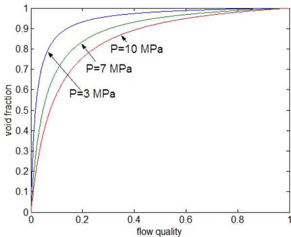
Figure 2. Effect of water pressure on  $\alpha$  vs x for S=1.
