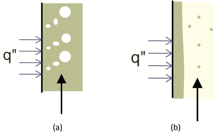
Figure 8. (a) Nucleate boiling (typical of bubbly and plug flow), (b) Forced evaporation (typical of annular flow).
