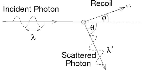
Figure 4.13: Compton scattering geometry in the scattering plane.
