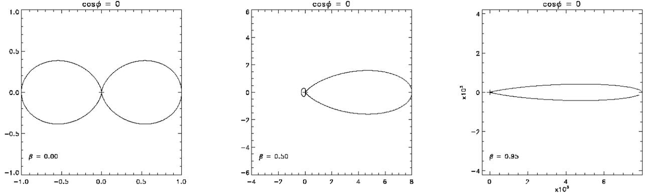
Figure 4.9: Polar plots of the radiation intensity as a function of direction, with acceleration perpendicular to  $\mathbf{v}$ , for the case where  $\hat{\mathbf{R}}$  lies in the plane of  $\mathbf{v}$  and  $\dot{\mathbf{v}} \wedge \mathbf{v}$ .
