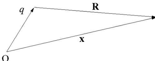
Figure 4.1: Vector coordinates of charge and field point.
