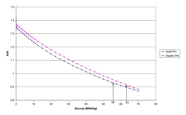
Figure 4: Keff versus In-Core Life for Solid and Duplex Fuel Pins
