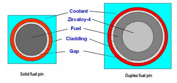
Figure 3: Duplex Fuel Pin Geometry
