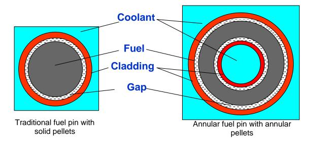
Figure 2: Annular Fuel Pin Geometry (Kazimi)
