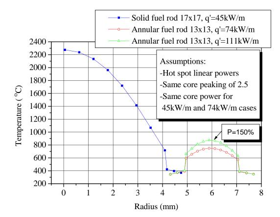
Figure 1: Solid/Annular Radial Fuel Temperature Profile (Kazimi)
