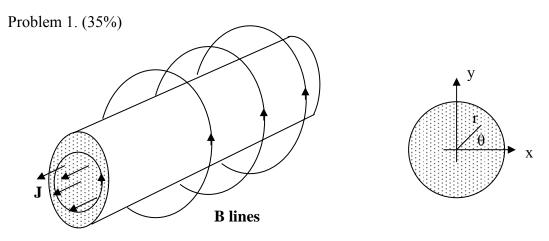
The figure depicts a long z-pinch with current density  $\vec{J} = \hat{z}J(r)$ , magnetic field  $\vec{B} = \hat{\theta}B(r)$ , and pressure p = p(r). There is no flow and the resistivity is assumed to be zero. Also  $n_e = n_i$ ,  $p_e = p_i$  and  $Z_i = 1$ .
