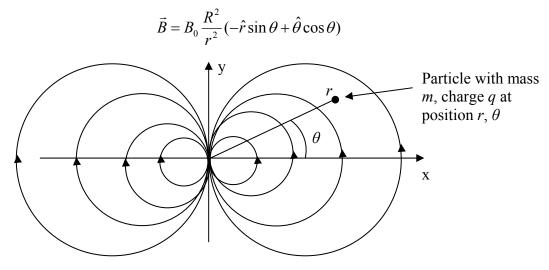
where *R* and  $B_0$  are constants and  $r, \theta$  are the usual cylindrical coordinates. The field is independent of the *z*-coordinate. Hint: The field lines for this 2-D dipole are circular and are given by  $r \alpha \cos\theta$ .
