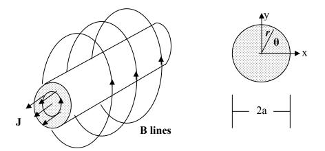
a) The plasma is undergoing rigid-body rotation in the  $\theta$ -direction, i.e., the plasma velocity is  $\vec{V} = \hat{\theta} r \Omega$ where  $\Omega$  is a constant. What is the relationship among B(r), p(r) and  $\Omega$  necessary to assure MHD equilibrium?
