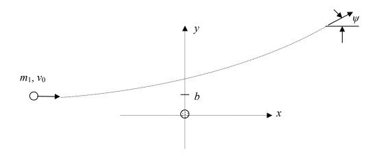
has infinite mass and is therefore stationary during the collision. The moving particle has mass  $m_1$ , speed  $v_0$  and the impact parameter for the collision is b.
