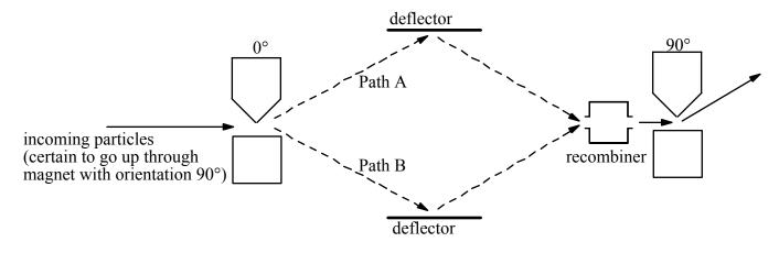
Suppose we set up the two-path experiment as shown above, with the incoming particles prepared in such a way that they are certain to go up through a magnet with orientation 90°. When we put particle detectors in Paths A and B, we find that any incoming particle activates one or the other of them. Hence we conclude:
