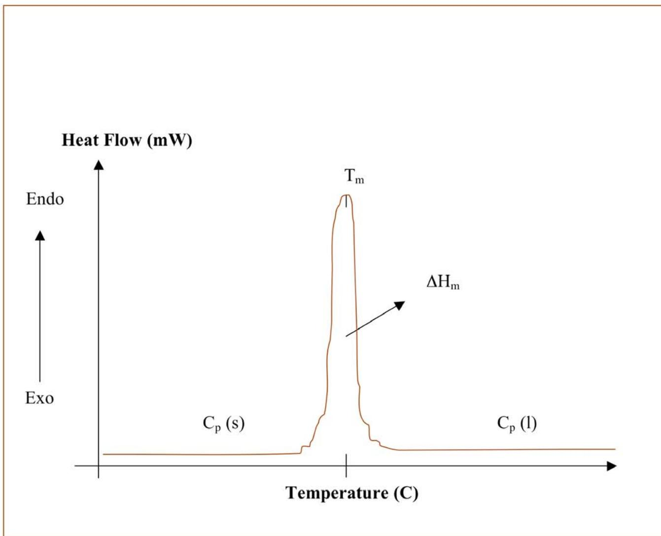
Figure 2: Schematics of a DSC thermogram, where  $C_p$  defines the heat capacity in the solid and liquid phase,  $T_m$  the melting temperature,  $\Delta H_m$  the enthalpy of melting or the latent heat of fusion. Note that heat absorbed is chosen positive (endothermic). [symbols as defined in 3.012 lecture notes]
