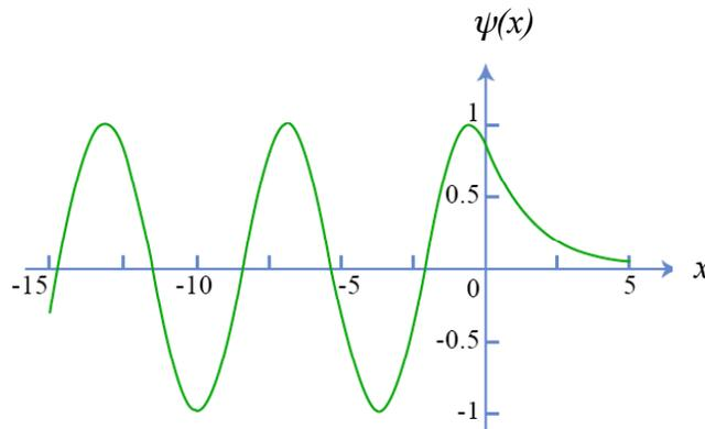
**Figure 2.** Wavefunction of an electron at the step-like potential (source: MIT OCW).
