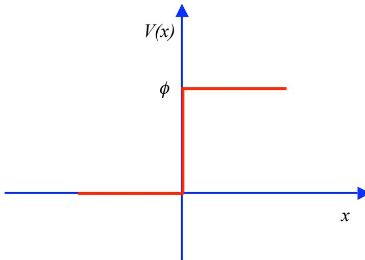
**Figure 1:** Step-like potential at the metal-vacuum interface.
