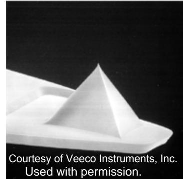
**Figure 2** An SEM micrograph of a typical AFM cantilever. (Veeco Instruments, <http://www.veecoprobes.com>)
