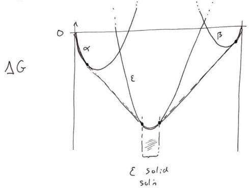
• Suppose that, instead of being a solid solution, the  $\epsilon$  phase is very intolerant of deviations from stoichiometry e.g.  $A_{1-n}B_n$ , n fixed
