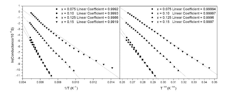
Near room temperature, mixed ionic and extended state conduction
