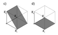
You might notice that some directions and planes in the crystal look the same: the atoms are spaced the same amount. This is due to symmetry in a crystal: for example, if you look down any of the diagonals in a cubic lattice, the atoms you "see" look the same! These equivalent directions and planes are called families. For example, the  $\langle 100 \rangle$  family of directions includes [100], [010], [001], [001], [010], and [001] in a cubic crystal.
