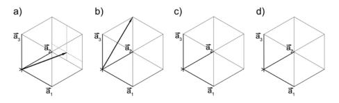
For a), we can see that the end of the vector is located at  $\frac{1}{2}\vec{a_1} + 1\vec{a_2} + \frac{1}{4}a_3$ . We can convert this to a crystallographic direction by multiplying through by 4 to get rid of the fractions while preserving the ratios. The direction shown in a) is therefore [241]. For b), the end of the vector is located at  $1\vec{a_2} + 1\vec{a_3}$ , which is represented as [011]. Finally, the [100] and [211] planes are shown below:
