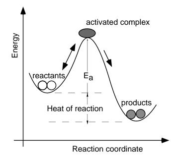
Figure 7 Schematic of a reaction via activated complex formation
