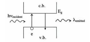
$$\lambda_{emitted} = \frac{hc}{E_g} = \frac{6.6 \times 10^{-34} \times 3 \times 10^8}{0.7 \times 1.6 \times 10^{-19}} = 1.77 \times 10^{-6} \text{ m}$$
