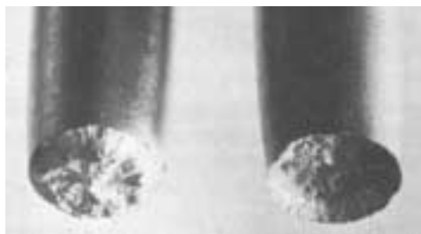
Figure 5: Cup-and-cone fracture in a ductile metal.
