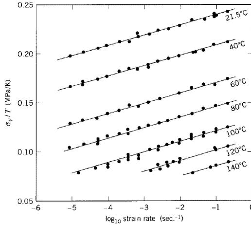
Figure 12: Eyring plot showing dependence of yield strength on temperature and strain rate in polycarbonate (from N.G. McCrum, C.P. Buckley and C.B. Bucknall, *Principles of Polymer Engineering*, Oxford University Press, 1988).
