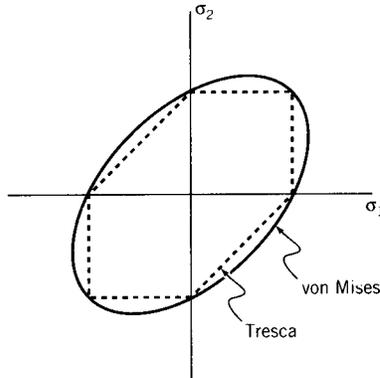
Figure 7: Yield locus for the von Mises criterion.
