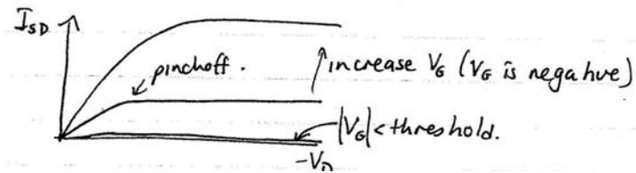
At threshold  $V_g$ , n goes into inversion and forms channel. Current  $I_{SD}$  flows, but channel is narrower near D, and eventually pinches off  $\rightarrow$  limits  $I_{SD}$ .
