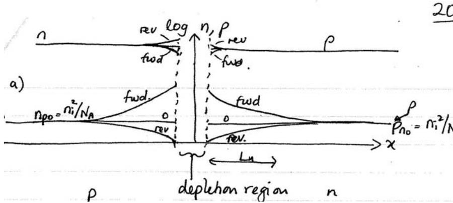
depletion region, decays away with characteristic length  $L_n$  (10s of  $\mu\text{m}$ ) slight reduction of electron concentration near depletion region of n side.
