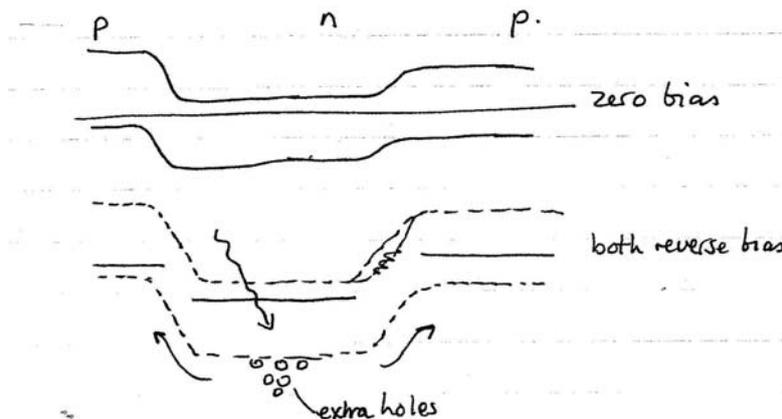
Note: Putting EB in fwd bias means a large current already flows through E→C, so the light-generated carriers would not add much to this.
