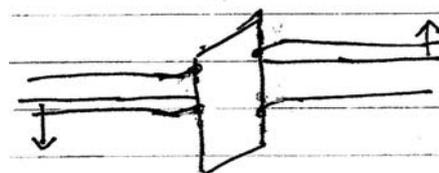
This 'unbends' the bands near the interface. Each side has less depletion than the unbiased case. A large bias could lead even to accumulation. Acts like a capacitor.
