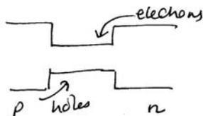
Also traps light due to change in refractive index (plus shiny sides of laser confine light). Also cladding doesn't reabsorb light since band gap larger.
