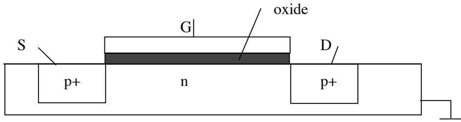
a) What happens when you apply a voltage  $V_G$  to G (when S and D are grounded)? Consider both positive and negative voltages. Illustrate with a sketch of the MOS band diagram.
