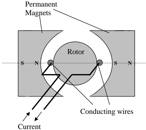
A sliding electrical contact reverses the polarity of the applied current when the rotor has reached 90 degrees from the position shown above.
