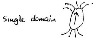
(Extra note - we didn't talk about this, but the elongated shape of the particles contributes to anisotropy because magnetism lies along long axis of particle.)
