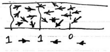
So bit size depends on *partilce size*. These are  $\approx 250\mu\text{m}$  long, so bit length will be at least  $1\ \mu\text{m}$ .
