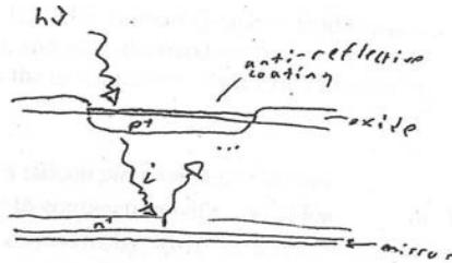
Considering optimal doping, we know that the i-region must be very lightly doped and the  $n^+$  and  $p^+$  regions must be heavily doped in order to completely deplete the i-region in equilibrium (more necessarily, in reverse bias).
