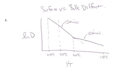
Diffusion mechanism is temperature dependent. At 150°, you are in extrinsic rather than intrinsic regime. Grain boundaries, defects increase rate of diffusion.
