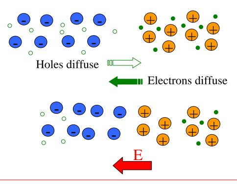
An electric field forms due to the fixed nuclei in the lattice from the dopants
