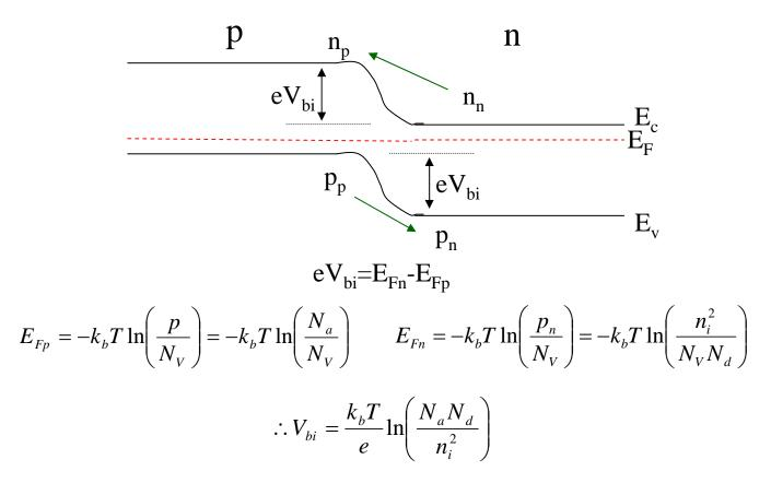
We can also re-write these to show that  $eV_{bi}$  is the barrier to minority carrier injection:
