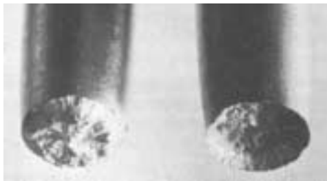
Figure 5: Cup-and-cone fracture in a ductile metal.
