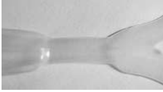
Figure 7: Necking and drawing in a 6-pack holder.
