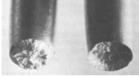
Figure 5: Cup-and-cone fracture in a ductile metal.
