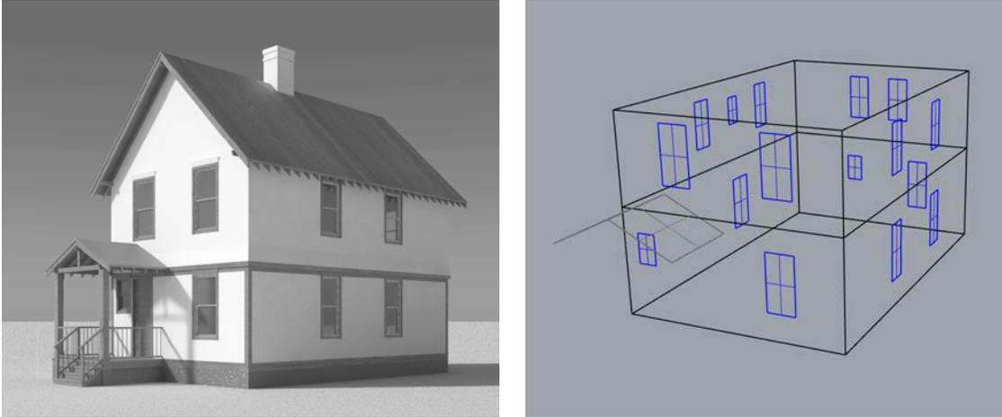
**Figure 1:** Daylighting (left) and two-zone thermal model of a residential house. The thermal model consists of breps for the two stories, individual surfaces for the windows that are co-planar with the walls and two surfaces that represent that porch roof.
