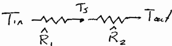
$$(T_{out} - T_s) = \frac{\hat{R}_2}{\hat{R}_1 + \hat{R}_2} (T_{out} - T_{in})$$
