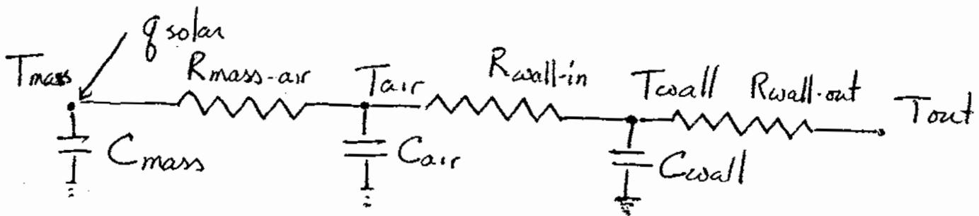
3 We use conservation of energy to write down one differential equation for each thermal capacitance
