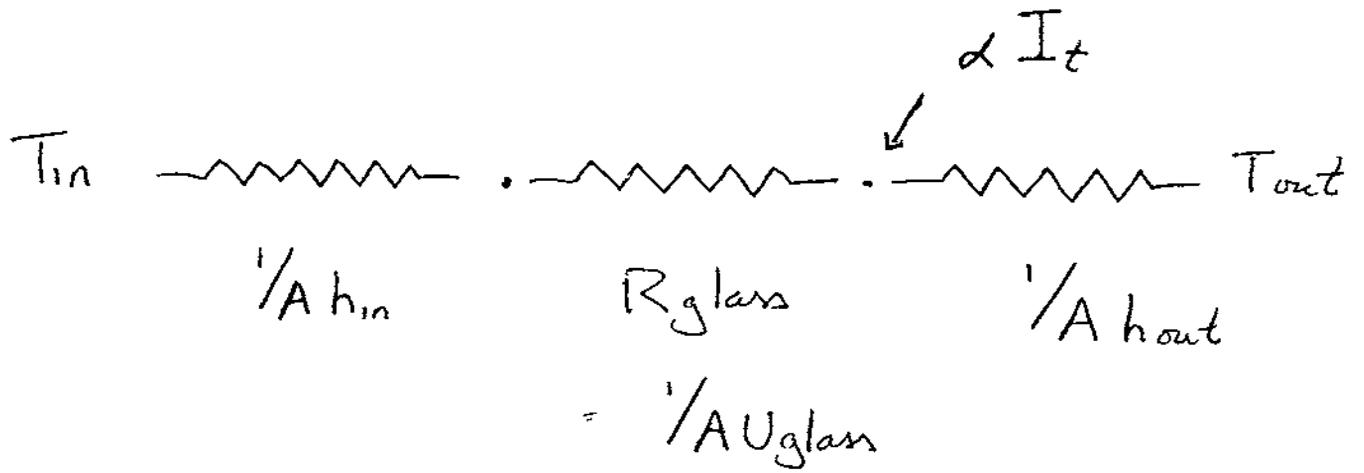
$$R_{window} = \frac{1}{A h_{in}} + R_{glass} + \frac{1}{A h_{out}} = \frac{1}{A U_{window}}$$
