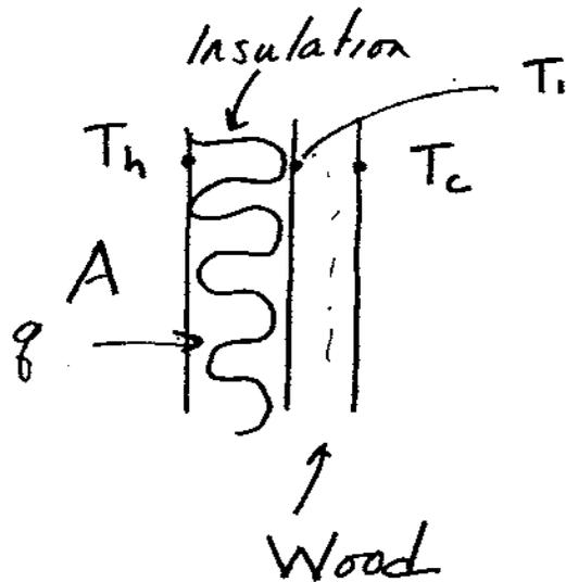
$$q = \frac{k_{\text{insulation}} A (T_h - T_i)}{L_{\text{insulation}}}$$
