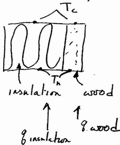
$$q = q_{\text{insulation}} + q_{\text{wood}}$$
