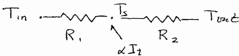
$$R_1 + R_2 = R_{wall} = \frac{1}{U_{wall} A}$$
