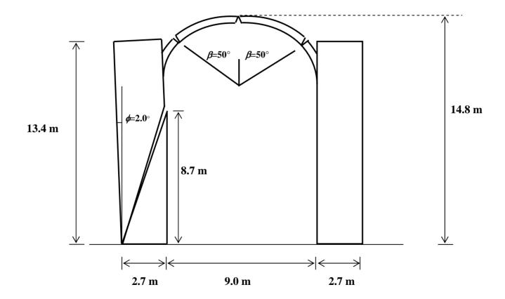
Collapse state of the church at Goa due to leaning of the South buttress. When the buttress has leaned outward by  $2^{\circ}$ , the thrust from the distorted vault will exceed the thrust capacity of the buttress and the vault will collapse. At this point, the crown of the vault has descended by 0.4 m and the thrust of the arch will have increased from 41 kN to 52 kN.
