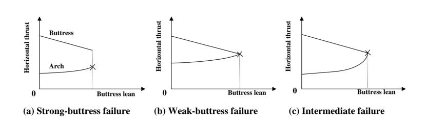
Three types of failure for an arch supported on leaning buttresses. The horizontal axis presents the inclination of the buttress and the vertical axis presents the change in horizontal thrust as the buttresses lean outwards. The arch collapse state is marked by "x".
