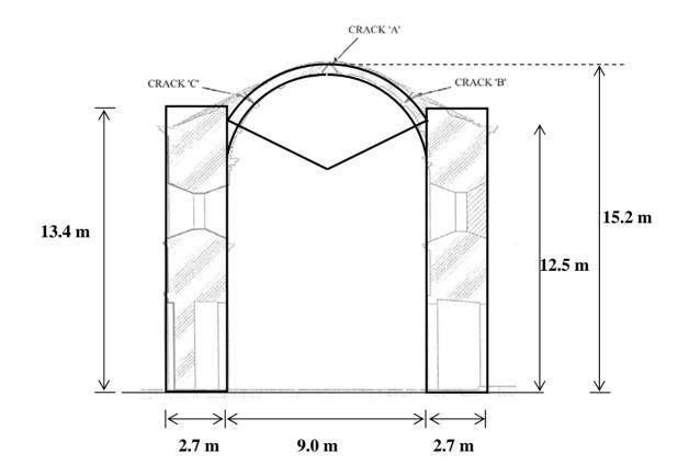
Unit weight of material 25 kN/m<sup>3</sup> – analyze 1 m strip
