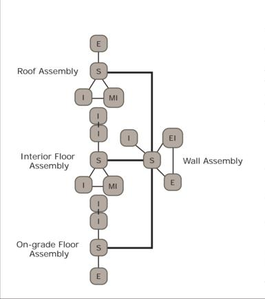
**Roof Assembly:** Roof structure and structural deck (S) Roofing (E) Ceiling (I) Lighting (MI) Wall Assembly: Wall structure (the support plus any lateral bracing, shear panels, or sheathing) (S) Exterior wall covering (EI) Windows and doors (EI) Interior wall covering (I) **Interior Floor Assembly:** Interior floor structure and floor deck (S)
