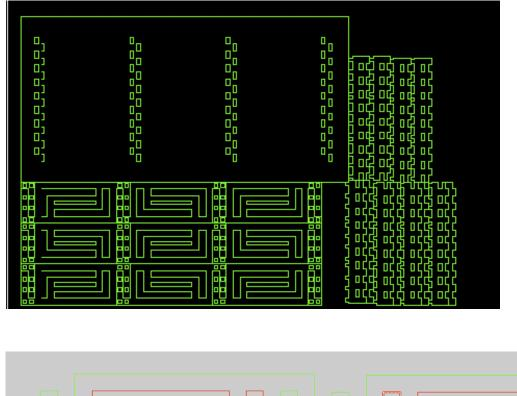
Tiles of rain screen evoke rectangular sections of colonial style siding. Right angle interlocking of tiles and variation between tiles adds interest.
